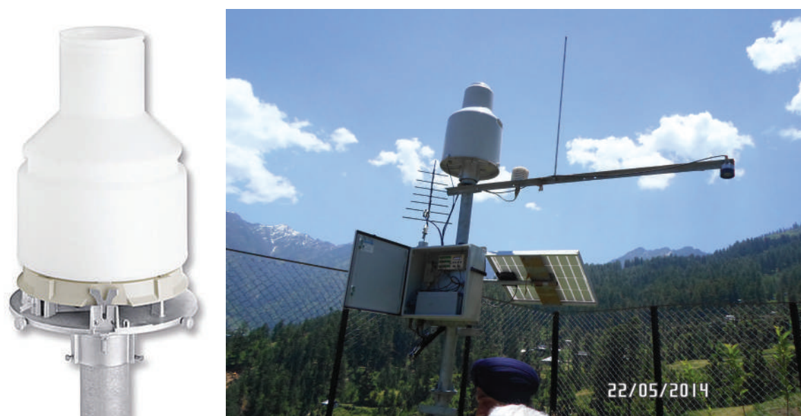
Figure 2.4: Frozen precipitation gauges: Pluvio 2 (left). A Pluvio installed in Madana, Himachal Pradesh, by Bhakra Beas Management Board (right)
