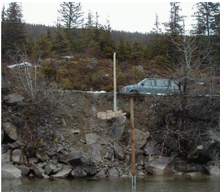
Figure 3.8: A staff gauge in two sections
