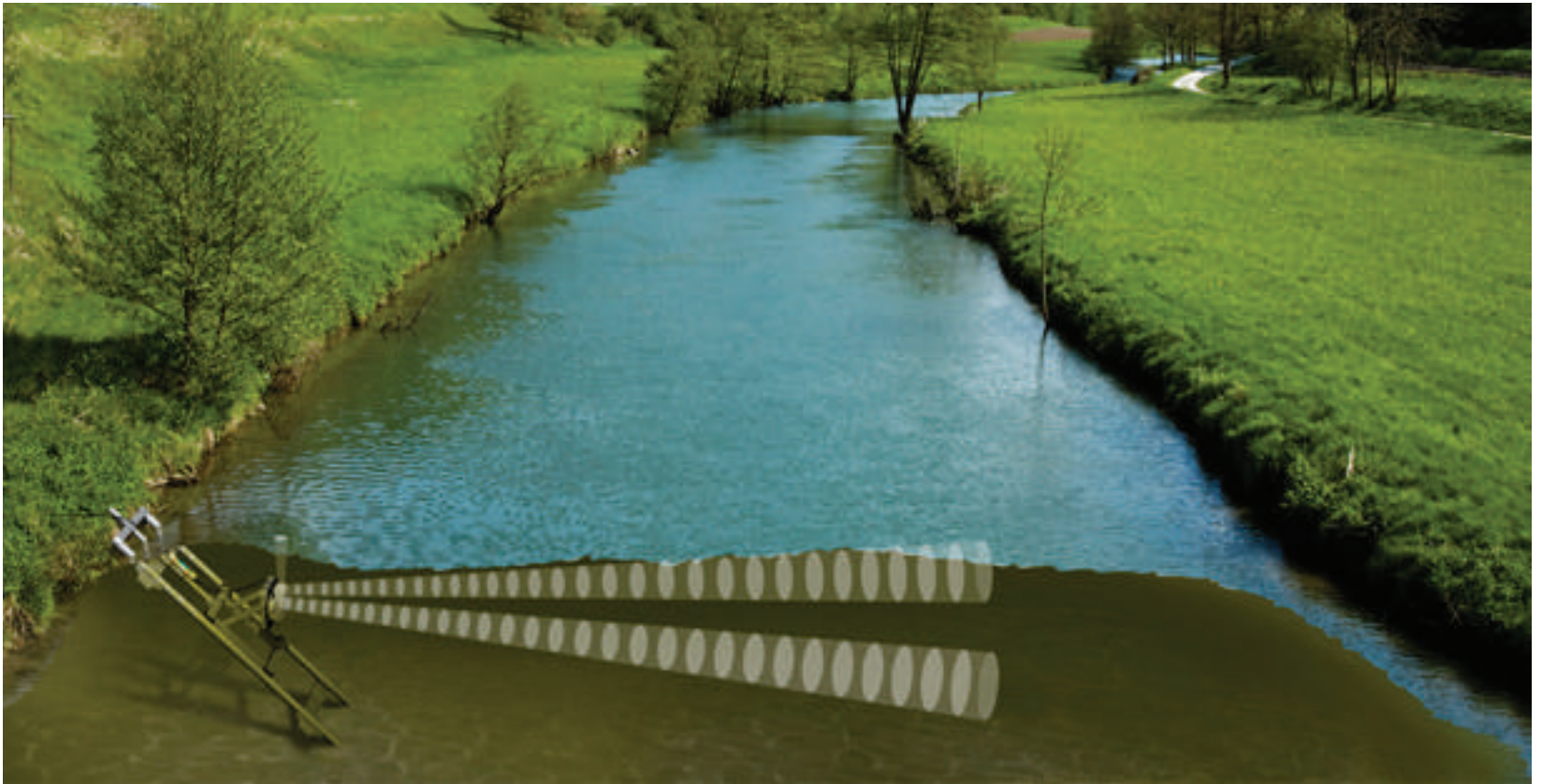
Figure 3.16: The application of a side-looking ADCP
