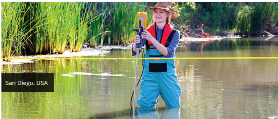
Figure 3.20: A hand-held acoustic Doppler velocity meter
