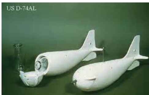
Figure 6.3: Depth-integrating suspended sediment sampler
