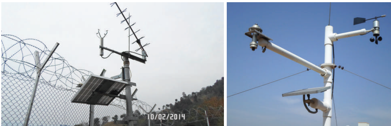
Figure 2.8: An ultrasonic wind velocity and direction sensor (left) and a cup-anemometer and wind vane-based wind velocity and direction sensor (right)
