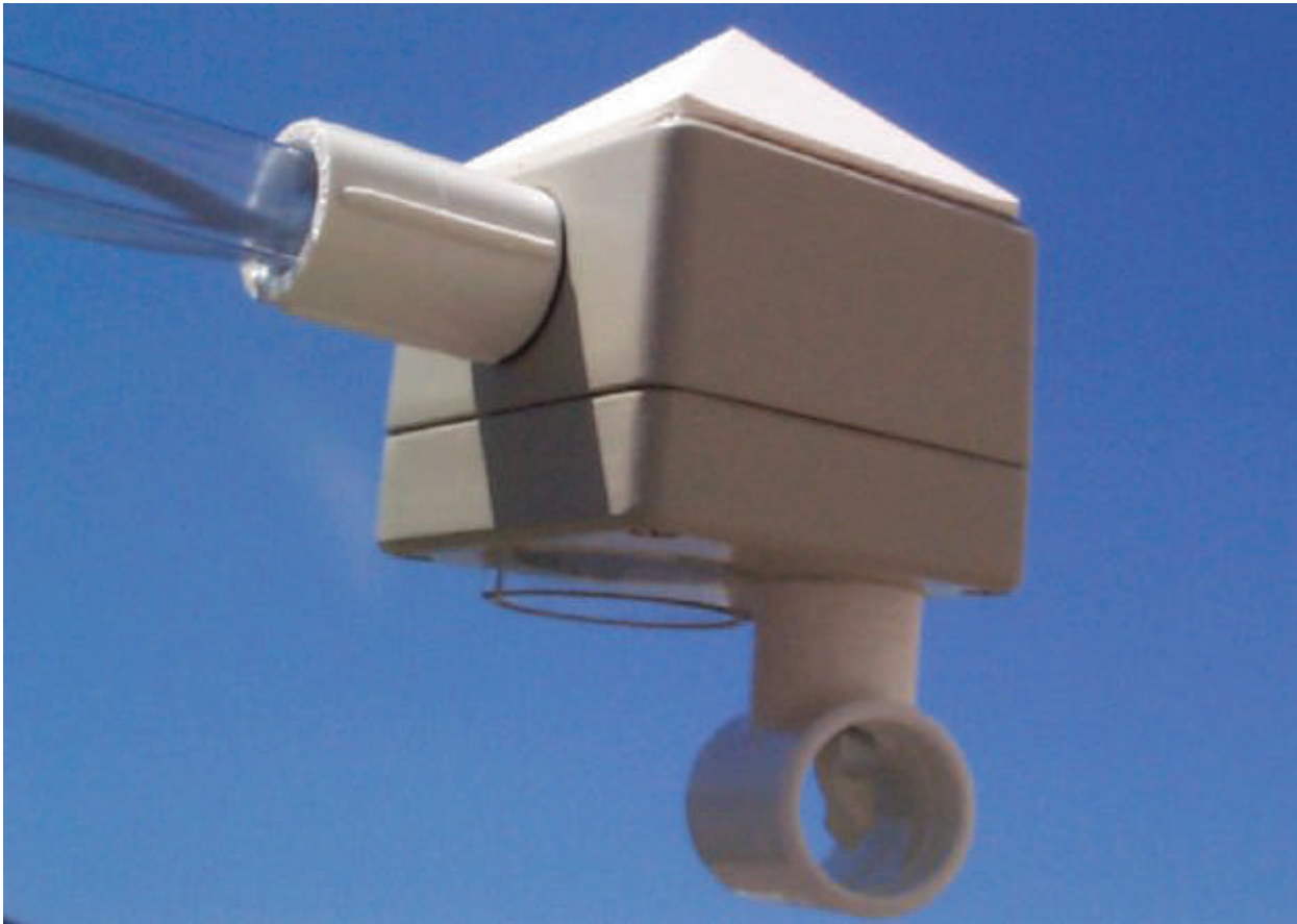
Figure 2.5. The Judd Communication snow depth sensor showing the temperature compensation device on the lower right and the ultrasonic sensor to the left of the temperature compensation device
