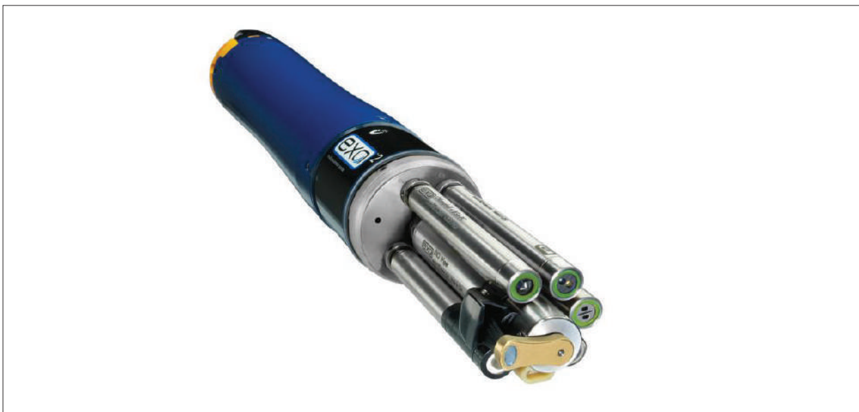
Figure 5.1: Multi-parameter water-quality sonde with sensors
