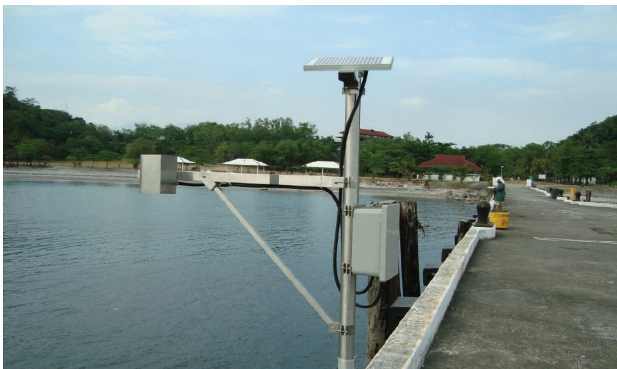
Figure 3.2: An ultrasonic sensor with boom mount
